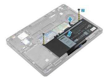
4. Unroute the cable from the routing channel [1] and remove the cable from the battery [2].
